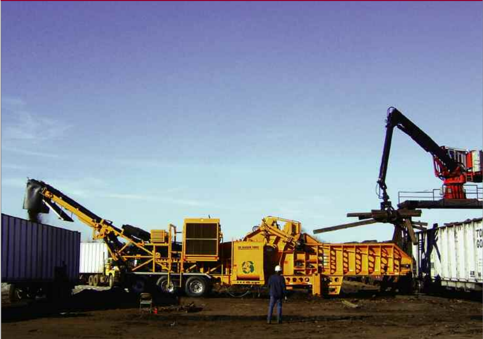
Snapped by Jason Feagans of National Salvage and Service Corp., this photo shows railroad ties being unloaded from railcars and loaded into a huge grinder.
